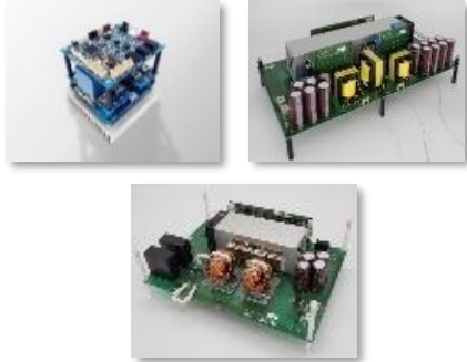
Bi-direction ACDC/DCDC reference board (Isolated/non-Isolated) with sample s/w
