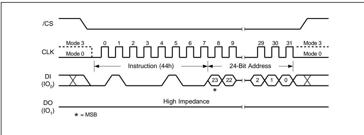
Figure 45. Erase Security Registers Instruction (SPI Mode only)
