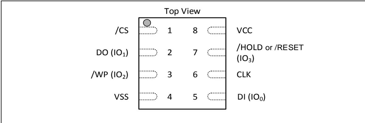
Figure 1b. W25Q16RV Pad Assignments, 8-pad WSON 6x5-mm, USON 2X3-mm (Package Code ZP, XH)
