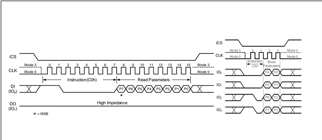
Figure 54. Set Read Parameters Instruction (SPI Mode Left/QPI Mode Right)
