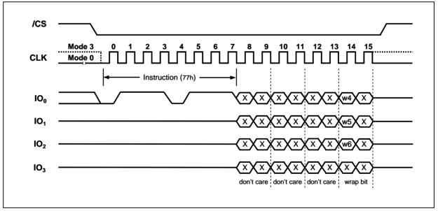
Figure 15. Set Burst with Wrap Instruction Sequence
