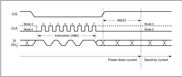
Figure 28a. Release Power-down Instruction Sequence
