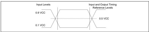
AC Measurement I/O Waveform
