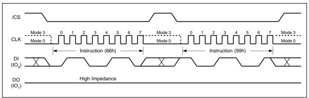
Figure 39a. Enable Reset and Reset Instruction Sequence
