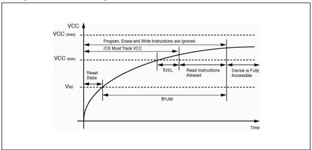
Figure 40a. Power-up Timing and Voltage Levels
