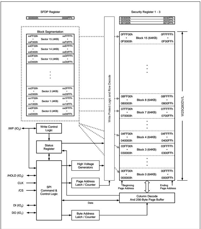
Figure 2. W25Q80DV/DL Serial Flash Memory Block Diagram
