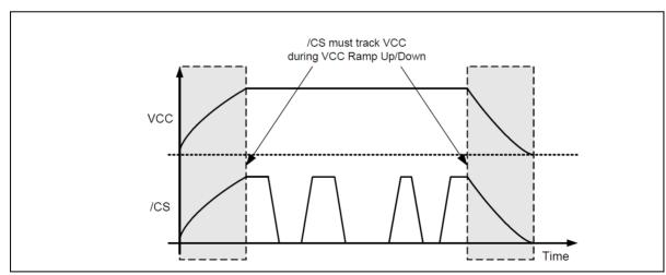
Figure 40b. Power-up, Power-Down Requirement
