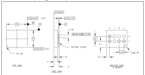
Note: Dimension b is measured at the maximum solder bump diameter, parallel to primary datum C.
