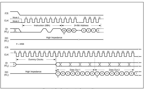
Figure 10. Fast Read Instruction Sequence Diagram
