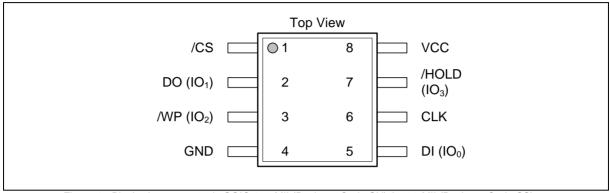
Figure 1a.Pin Assignments, 8-pin SOIC 150-MIL(Package Code SN) & 208-MIL(Package Code SS)
