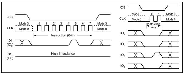
Figure 6. Write Disable Instruction Sequence Diagram
