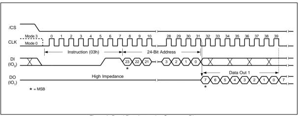
Figure 9. Read Data Instruction Sequence Diagram
