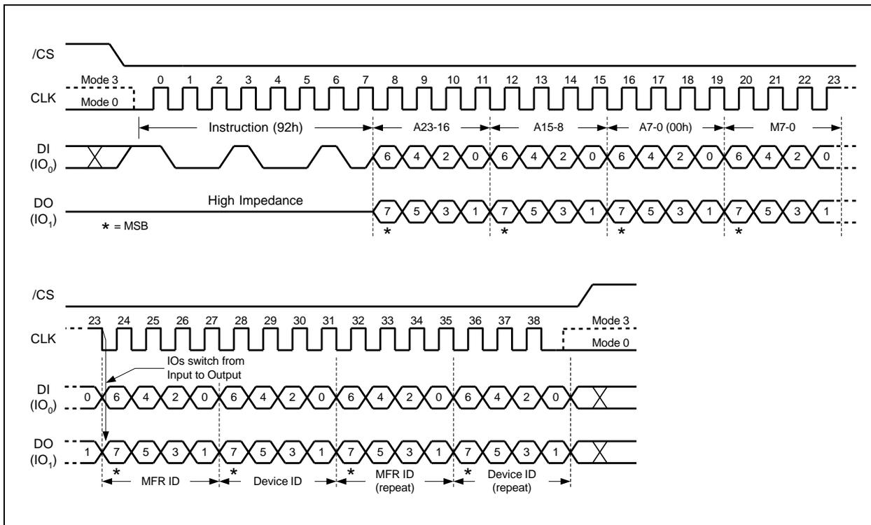
Figure 29. Read Manufacturer / Device ID Dual I/O Instruction
