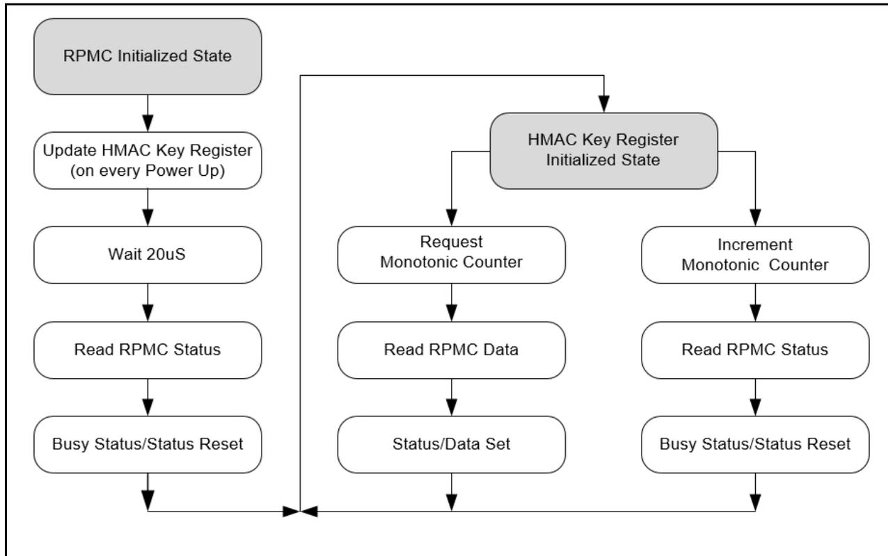
Figure 3b. W25R128JV RPMC Operation Flow Diagram
