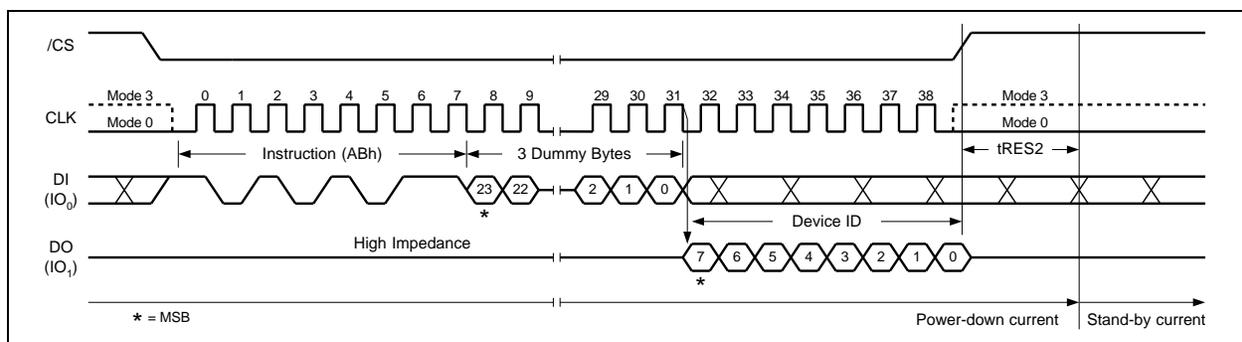
Figure 27b. Release Power-down / Device ID Instruction
