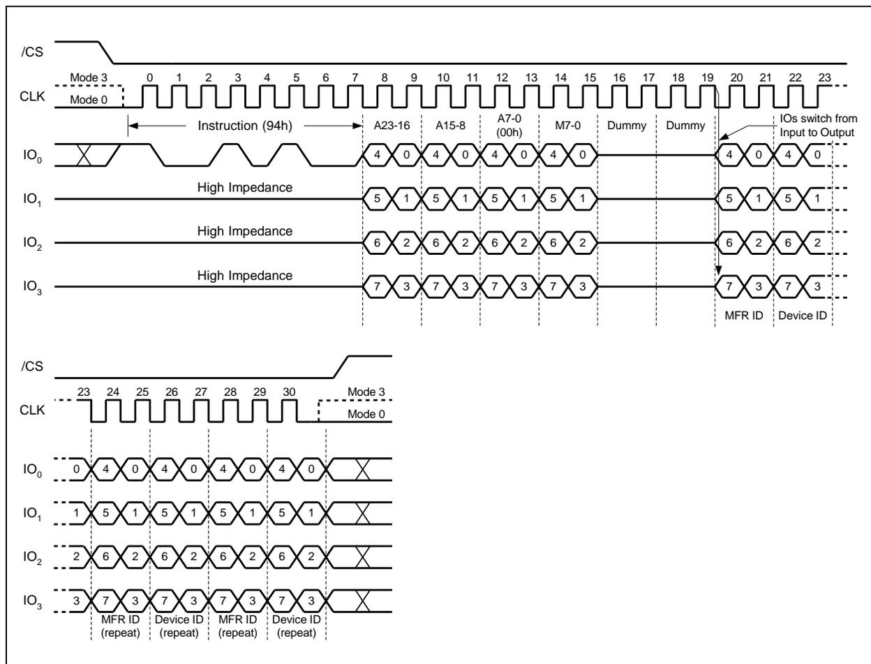
Figure 30. Read Manufacturer / Device ID Quad I/O Instruction
