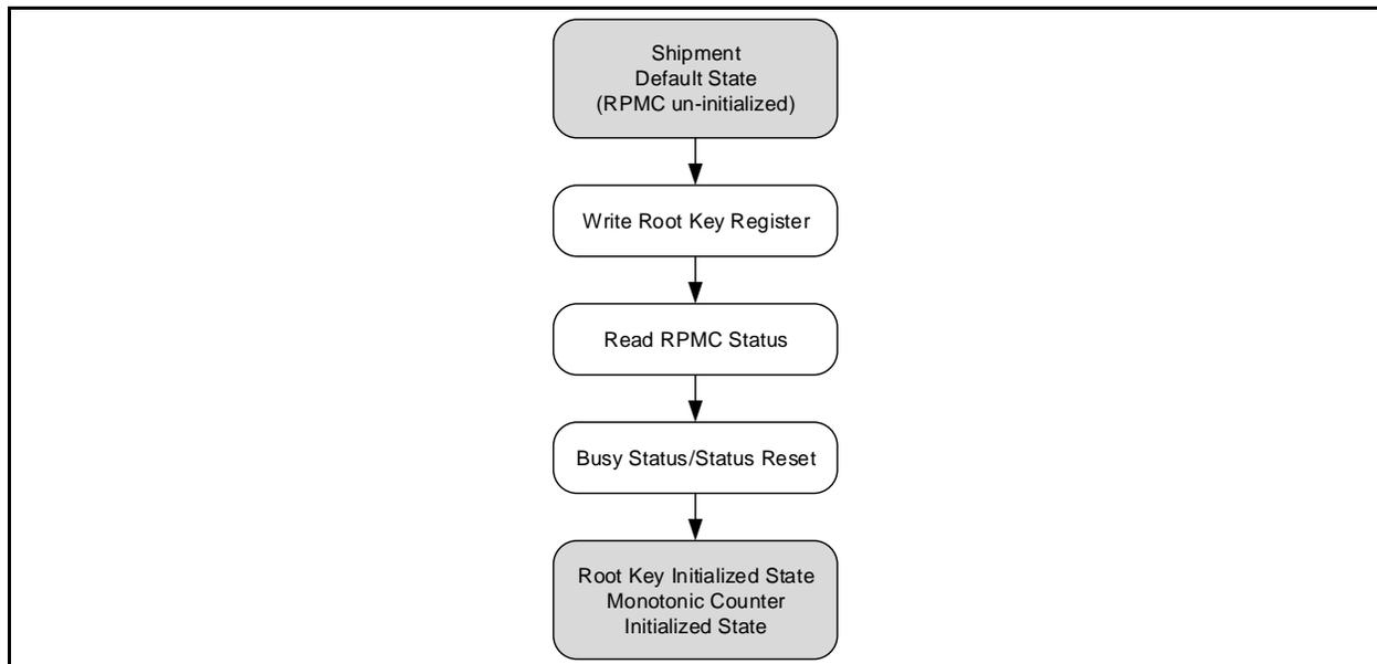
Figure 3a. W25R128JV RPMC Initialization Flow Diagram
