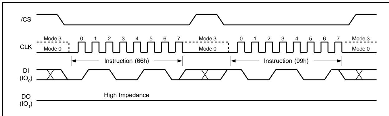
Figure 42. Enable Reset and Reset Instruction Sequence
