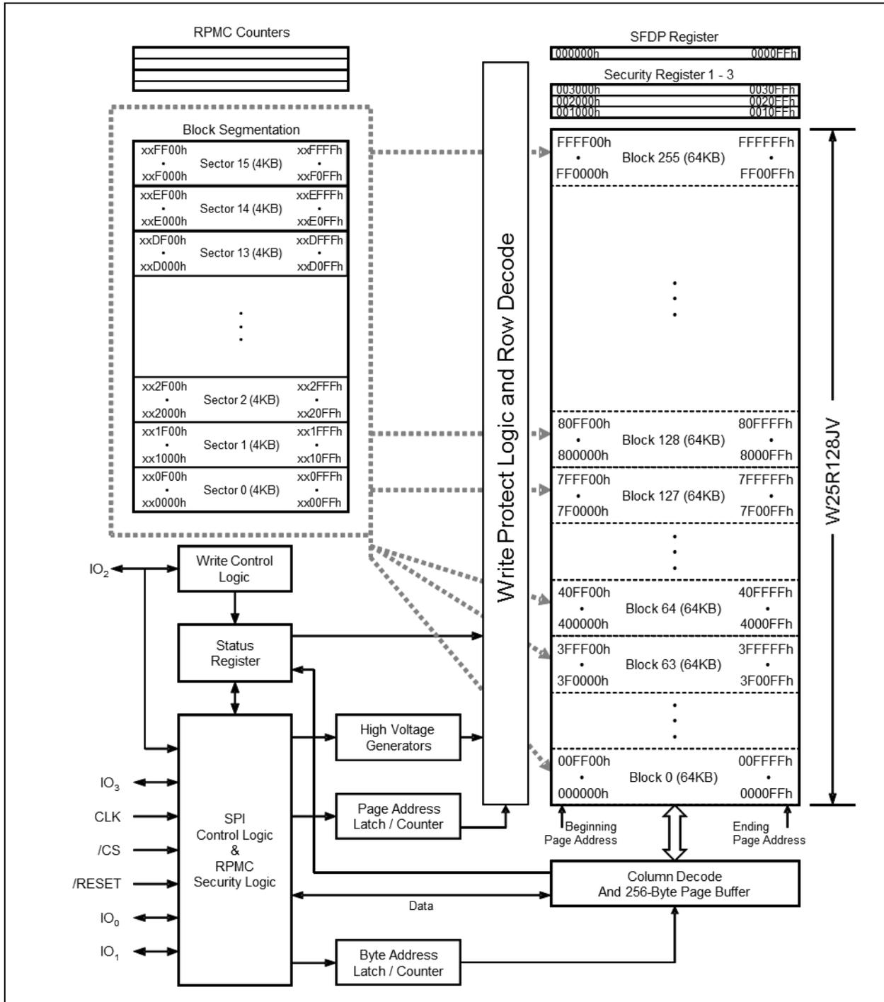
Figure 2. W25R128JV Serial Flash Memory Block Diagram
