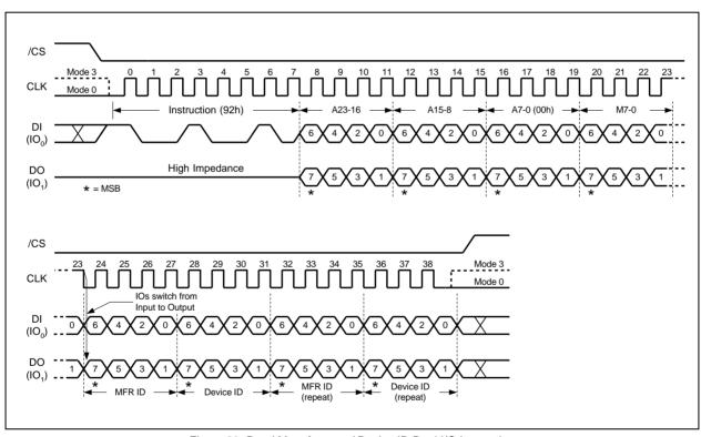
Figure 29. Read Manufacturer / Device ID Dual I/O Instruction
