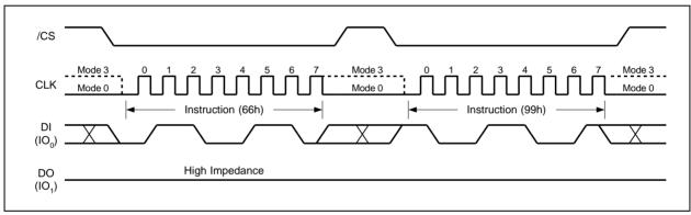
Figure 42. Enable Reset and Reset Instruction Sequence
