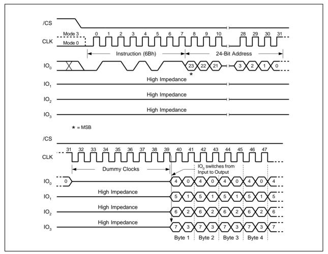
Figure 14. Fast Read Quad Output Instruction
