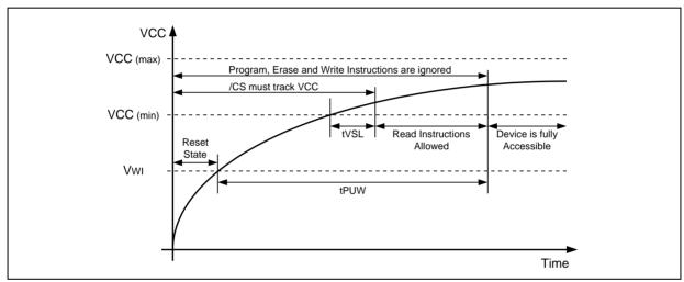
Figure 48a. Power-up Timing and Voltage Levels
