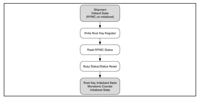
Figure 3a. W25R128JV RPMC Initialization Flow Diagram
