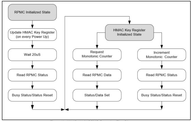
Figure 3b. W25R128JV RPMC Operation Flow Diagram
