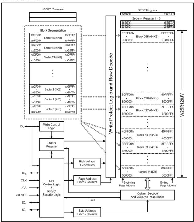
Figure 2. W25R128JV Serial Flash Memory Block Diagram
