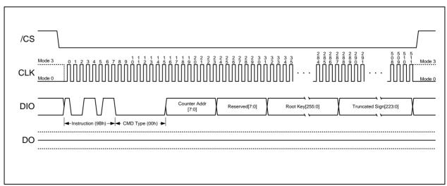
Figure 43. Write Root Key Register Instruction
