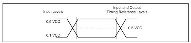
Figure 49. AC Measurement I/O Waveform
