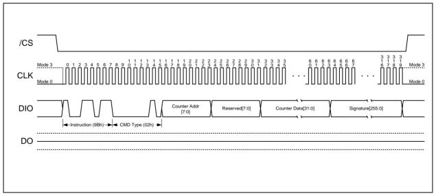
Figure 45. Increment Monotonic Counter Instruction
