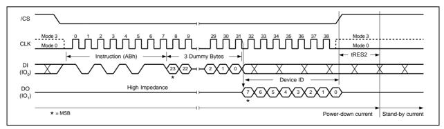
Figure 27b. Release Power-down / Device ID Instruction
