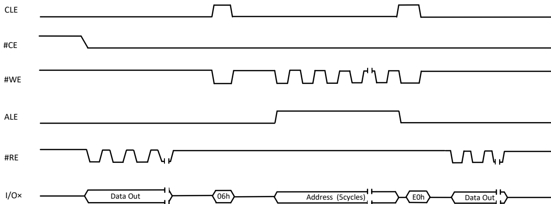
Figure 9-4 Two Plane Random Data Read (06h-E0h) Operation
